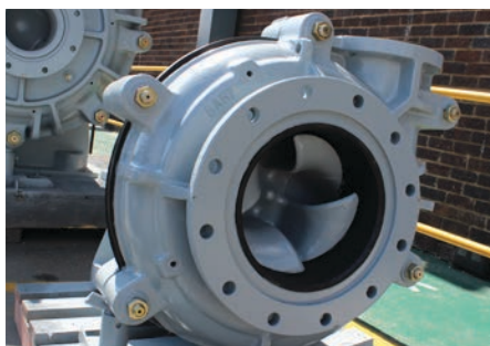
Top: Warman® AHF Froth Pump with Continuous Air Removal System (CARS)
